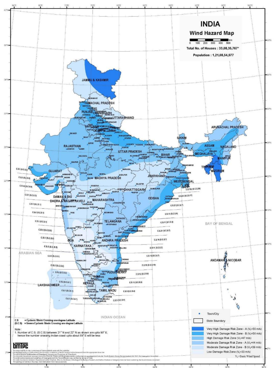
BMPIC - Vulnerability Atlas- 3rd Edition; Peer Group, MoHUA; Map is Based on digitised data of SOI, GOI; Basic Wind Speed Map National Building Code: 2016; Cyclone Data, 1951-2015, IMD, GOI; Houses/Population as per Census 2011; Houses including vacant & locked houses. Disclaimer: The maps are solely for thematic presentation.
