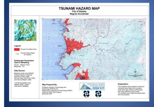
Basis of listing of Tsunami Prone Barangays are indicative maps utilizing maximum wave height and inundation (worst case scenario earthquakes) from major offshore source Modeling results using Rapid Earthquake Damage Assessment System (REDAS) Software based on empirical equations
