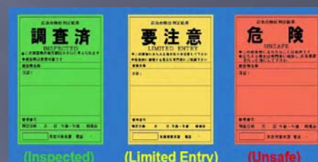
BRI disaster response – building assessment
