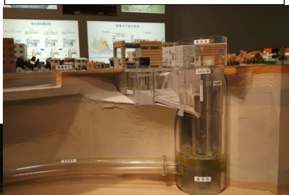
Model showing Kanda River Underground Regulating Reservoir Tunnel
