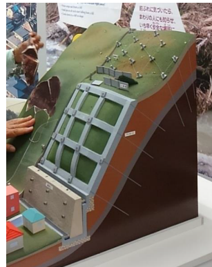
Model showing Sediment Disaster Prevention using Anchor work in Nigawa Landslide Museum (B) Sediment disaster countermeasures in Tamba city
