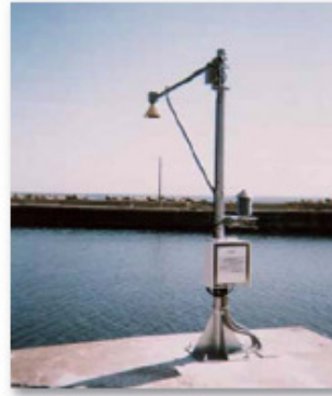
◆ Acoustic Type Gauge Station
