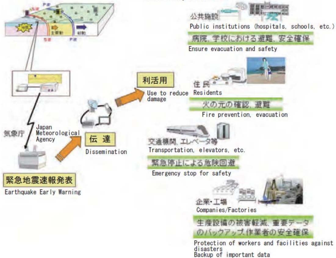
Figure 3.4 Outline of Earthquake Early Warning Information Source: Cabinet Office, Government of Japan
