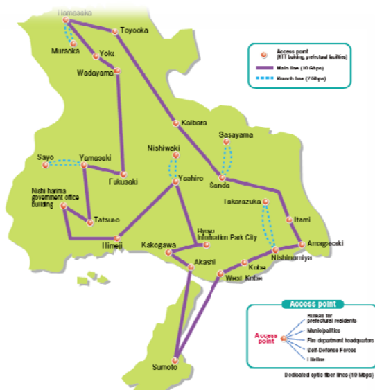
Network Construction of Hyogo Information Highway
