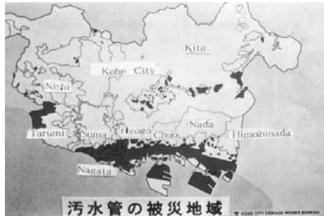
Map of damaged sewage channels (shaded areas)
