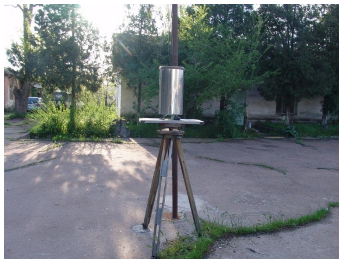
Fig. 72. Electronic rain gauge (Japan).
