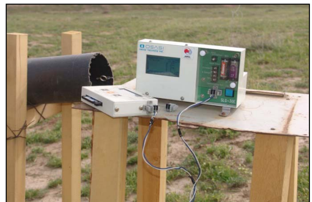
Fig. 70. Landslide displacement measurement with an automatic electronic extensometer.
