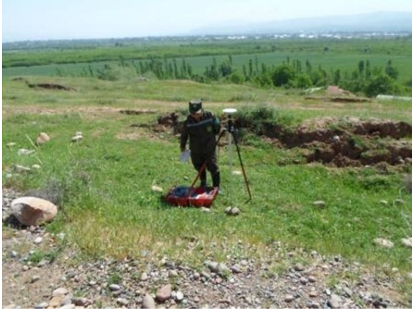
Fig.68. GPS receiver to measure Landslide displacement
