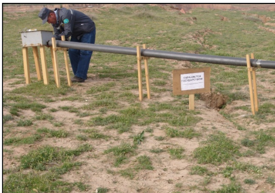
Fig. 70. Landslide displacement measurement with an automatic electronic extensometer.
