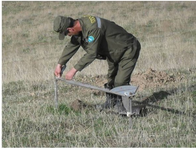
Fig. 71. Measurement disclosure landslide cracks using extensometer (SLD).
