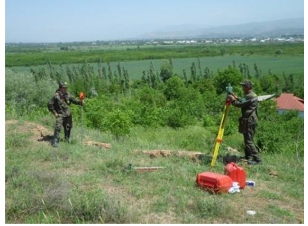
Fig. 69. Electronic tachymeter for shooting landslide
