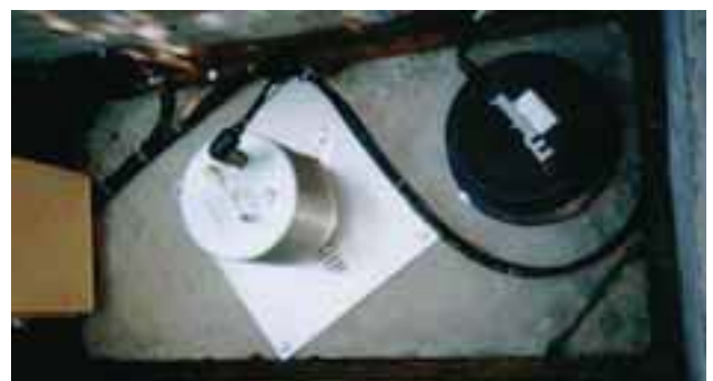
Fig. 29. Seismometer and Seismic Intensity Meter in Box
