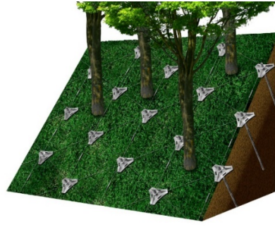
Reinforcement solutions against landslide by metal rock anchor combined with planting tree, grass on the slope
