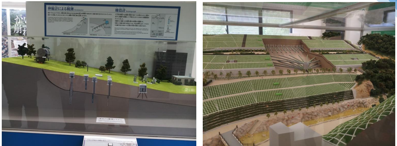
Figure 23: Model showing (A) Sediment Disaster Early warning system using "Inclinometer" in Nigawa Landslide Museum (B) Sediment disaster prevention using "Drainage works"
