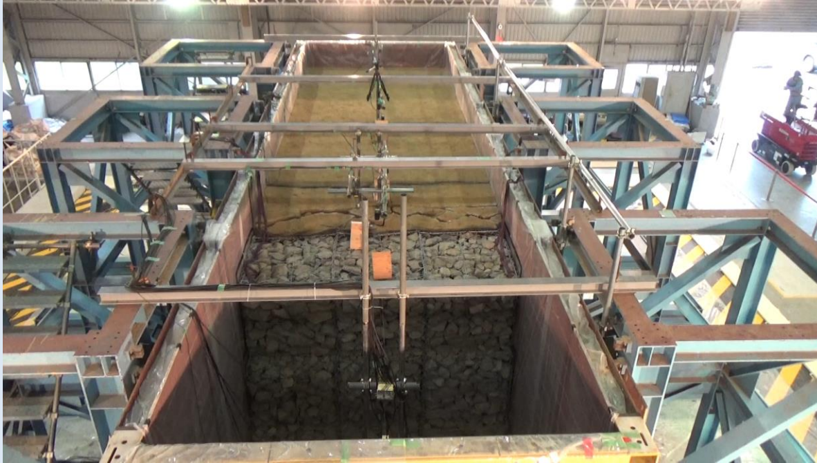
Case 2: Step wise-type Sinusoidal wave 3Hz (313Gal in fourth stage)
