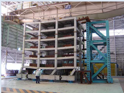
One-third (1/3) scale reinforced concrete building
