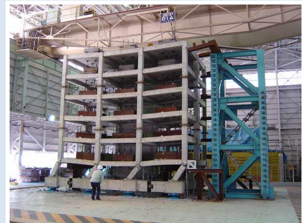
Observation of model's collapse process
