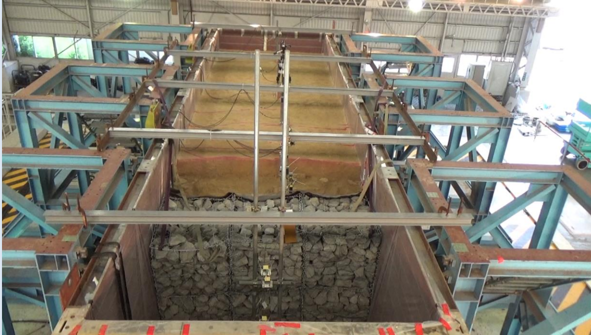
Case 1: Vertical-type Sinusoidal wave 3Hz (257Gal in fourth step)
