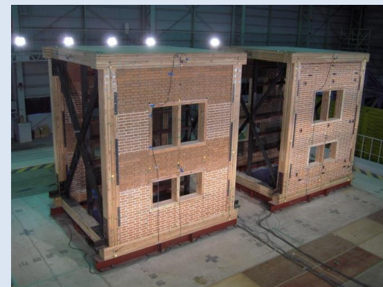
Wooden-frame brick structure
