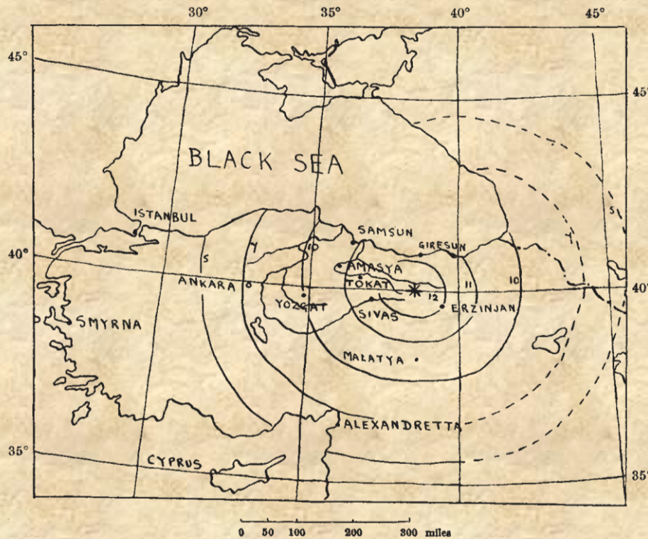
SKETCH MAP SHOWING THE APPROXIMATE EPICENTRE AND ISOSEISMAL LINES (MODIFIED MERCALLI SCALE OF 1931) OF THE ERZINCAN EARTHQUAKE OF DECEMBER 27, 1939.
