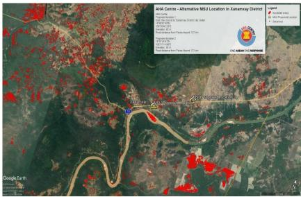
Overlay of Inundation Areas for determining location of Mobile Storage Unit
