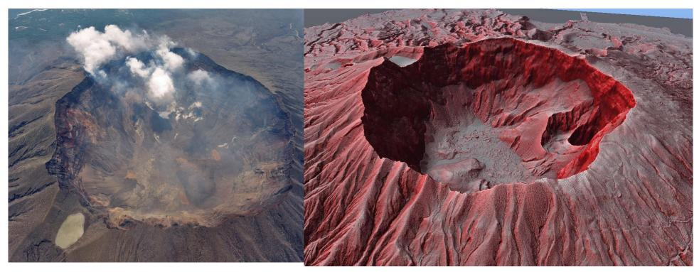
Mt. Miyakejima, Aerial photograph from Asia Air Survey Co., Ltd. Mt. Miyakejima, Red Relief Image Map produced from 1m LiDAR DEM by GSI, Japan
