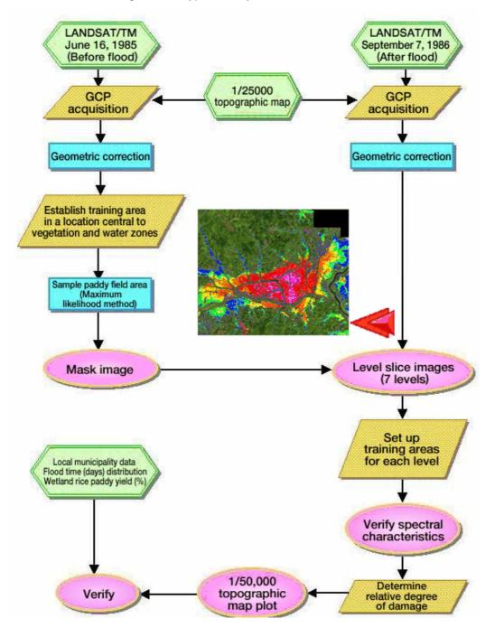
Fig. 3-6-3 Typical Analysis Process Flowchart
